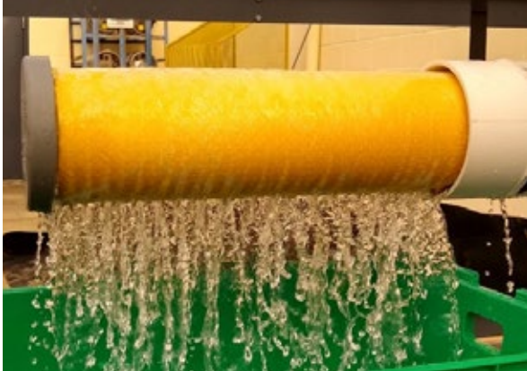
HFF removes hydrocarbons as it filters and processes water
