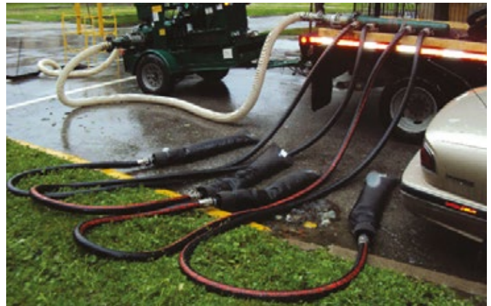
Multiple EVACs can be used with larger pumps with a multi-port manifold.
