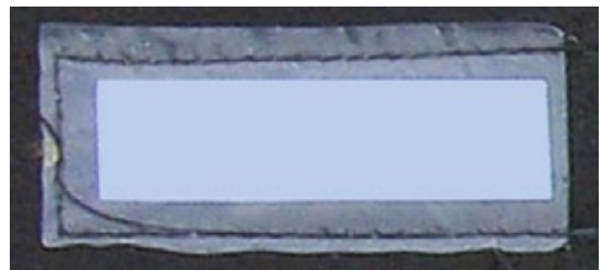
Hydrocarbon Detection Strip placed against outer skin.
