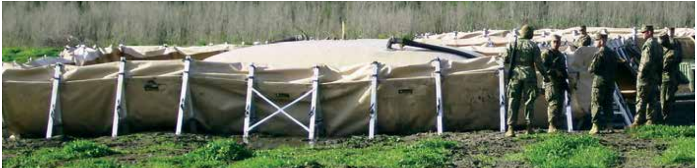
Field application of the All-Terrain Berm™ containing a flexible fuel tank. The All-Terrain Berm™ can be field-deployed by five people in 45 minutes on rough terrain. The individual aluminum A-frames enable the unit to adapt to the contour of the ground.
