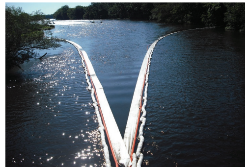
Sheen Boom (orange) deployed on the Kalamazoo River during the Enbridge Oil Spill (August 2010).
